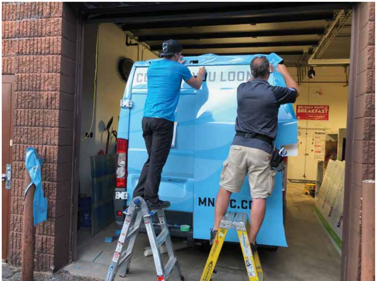
Installing Wrap Vinyl
